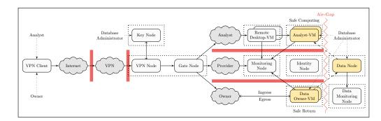
Figure 1 The multiple security layers in our reference implementation. Components in golden color contain sensitive data anytime, red bars are restricted firewall barriers. Dotted boxes denote physical servers on which nodes can be deployed or virtualized (the VPN Node and Gate Node can share a physical server).
