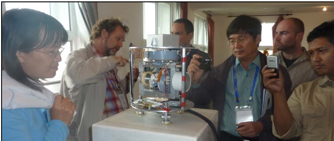
Figure 5. Demo of the AUTODIF MKII in the Changchun magnetic observatory absolute house.
