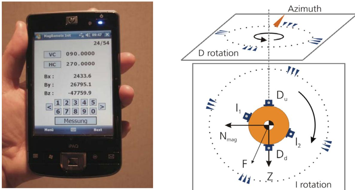
**Figure 1.** The PDA guiding through the measurement procedure (left) and a schematic illustration of the measurement positions (right)
