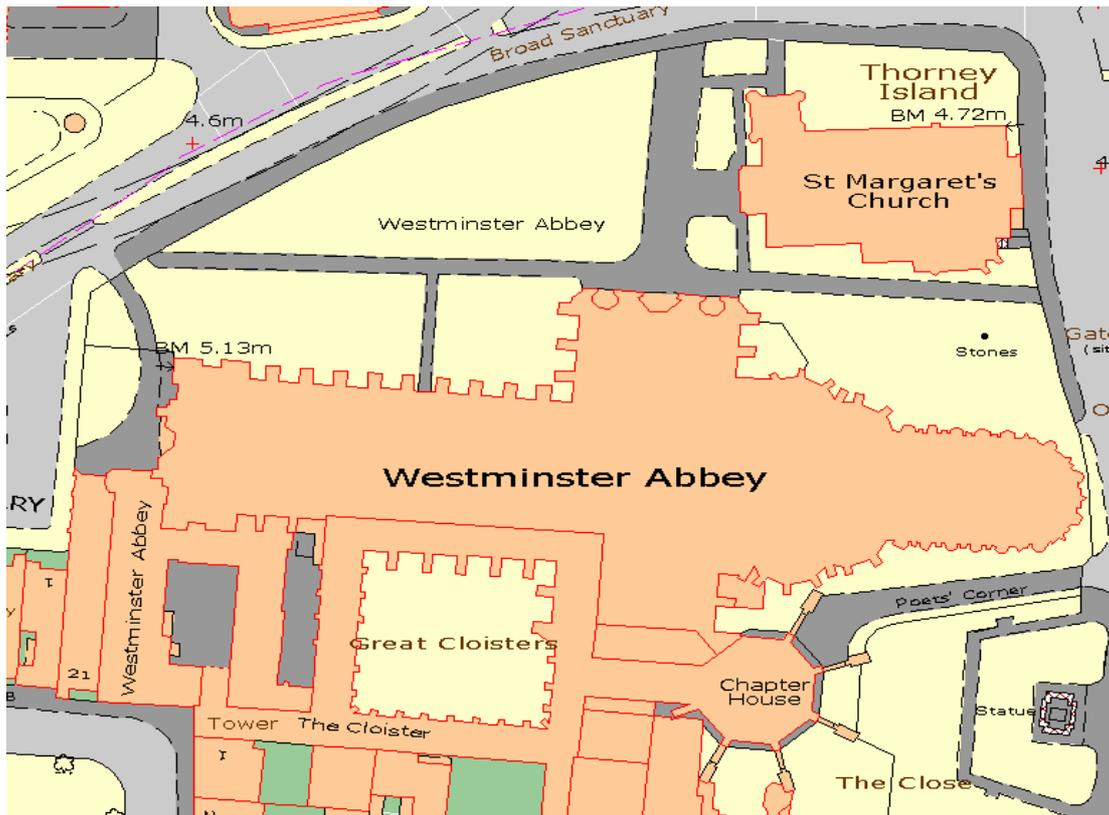
**Figure 2.** An extract of OS MasterMap, Topographic layer and selected themes of Westminster Abbey, London. Each feature, whether it is a point, line or area feature, has its own unique identifier known as a TOID onto which users can link and reference their own information.
