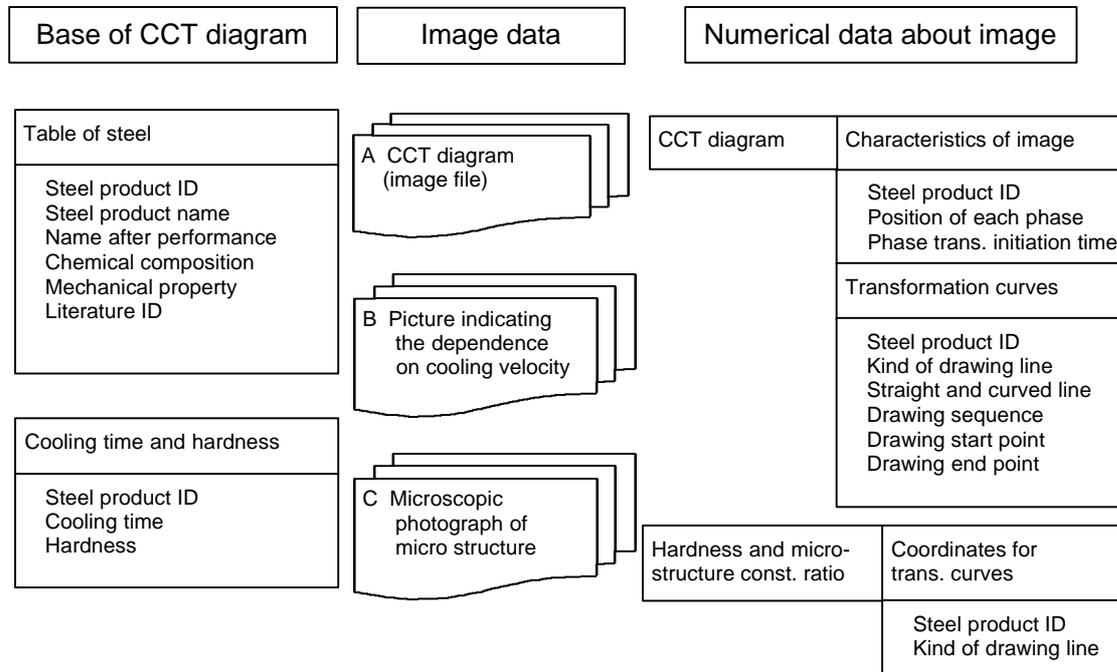
Figure 3. Data structure of a CCT diagram database
