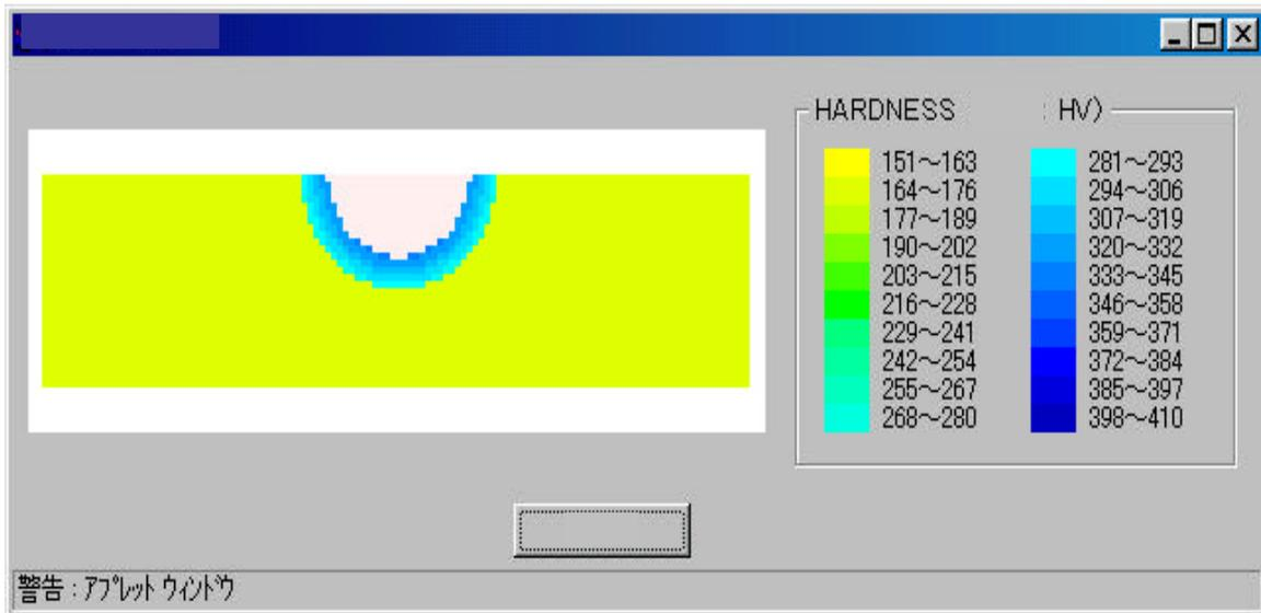
Figure 10. Contour lines of hardness through a cross-section of a weld.
