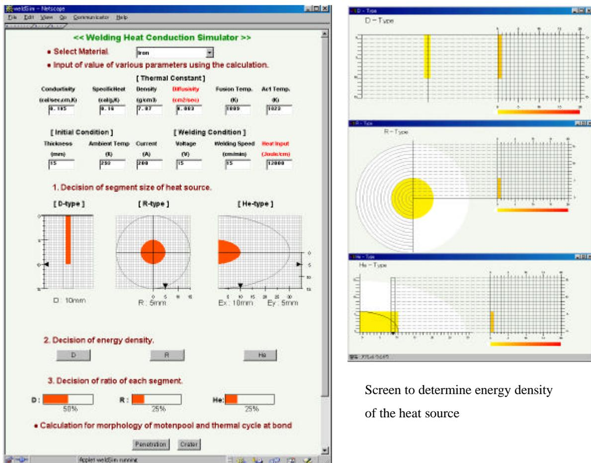
Screen to determine energy density of the heat source
