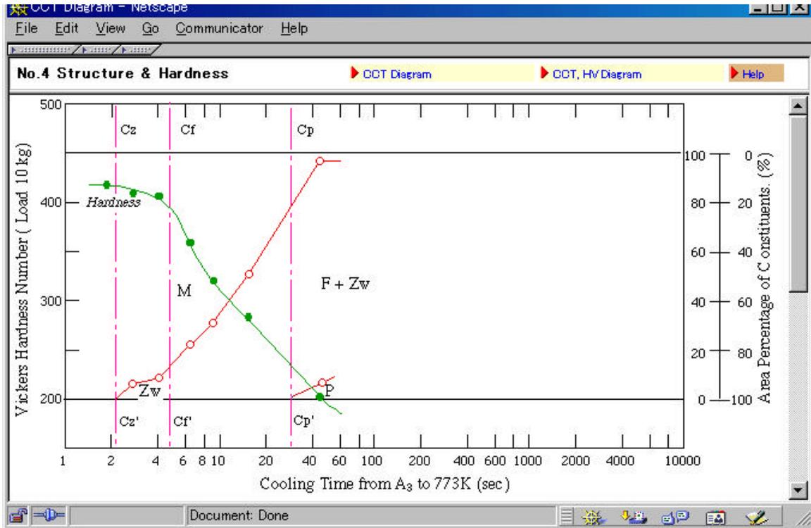
Figure 9. Changes in Vickers' hardness and the ratio of micro-structural constitutions with cooling time from the Ac<sub>3</sub> transformation temperature to 773 K.
