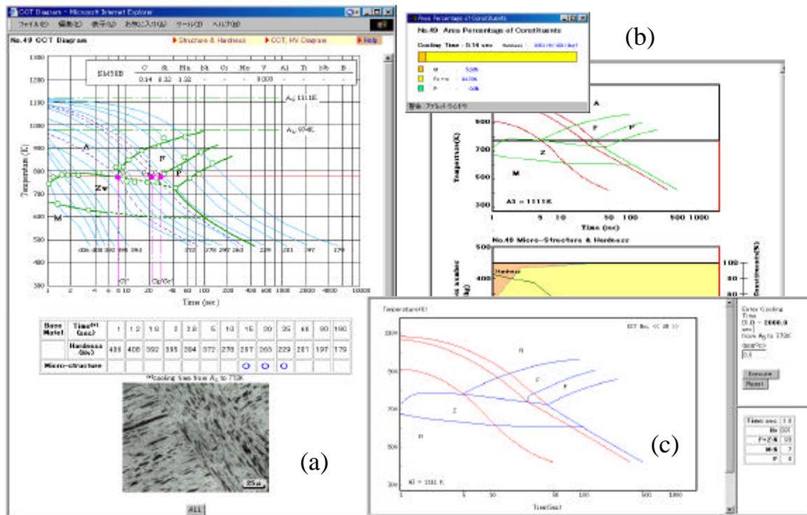
**Figure 4.** An example of the retrieval results from the CCT diagram database. (a) the original CCT diagram expressed as graphical data (b) the diagram recomposed interactively from numerical data and (c) another representation of the retrieved numerical data.
