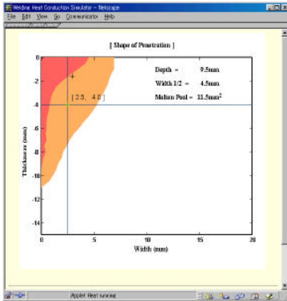
**Figure 6.** Shape of the molten pool and the HAZ.
