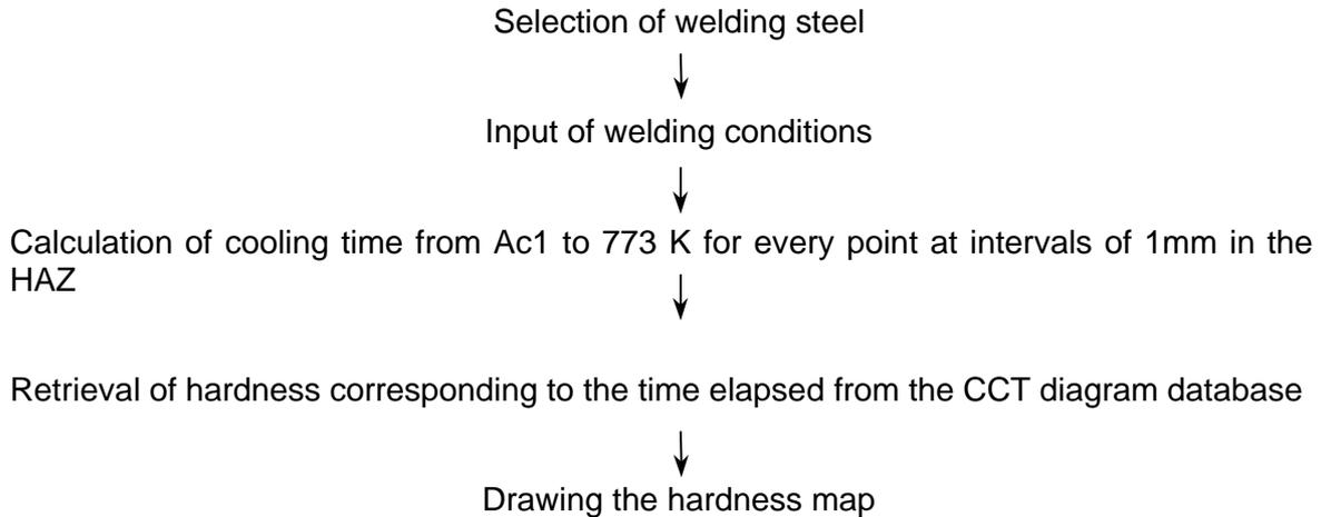
**Figure 8.** Flow-chart for the prediction of weld HAZ properties.
