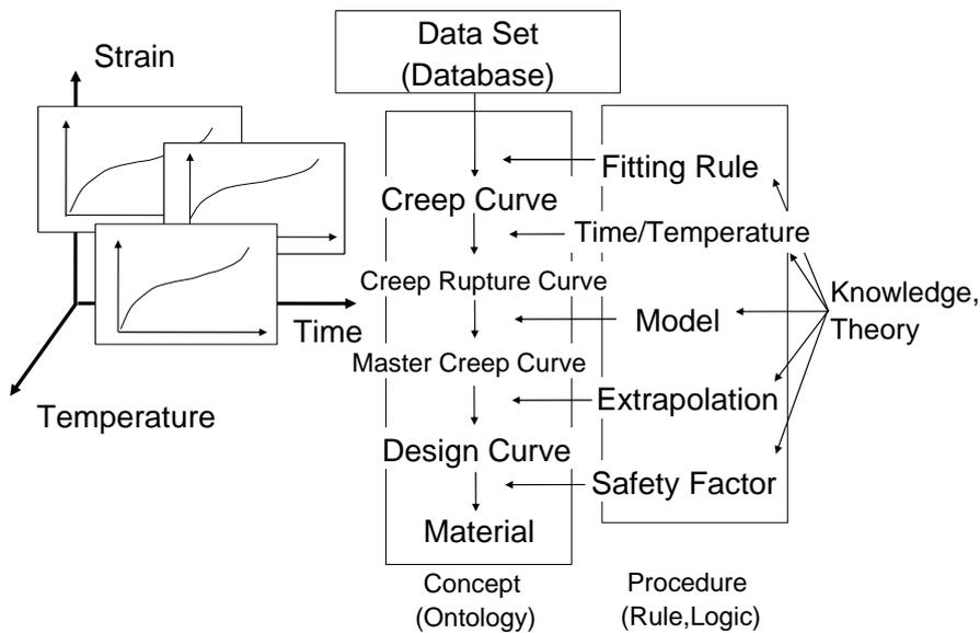
**Figure 7.** A flow of creep data analysis with Ontology and Rule
