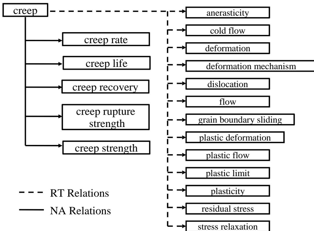
Figure 3. Entries in a metallurgical thesaurus relate to the entry “Creep”
