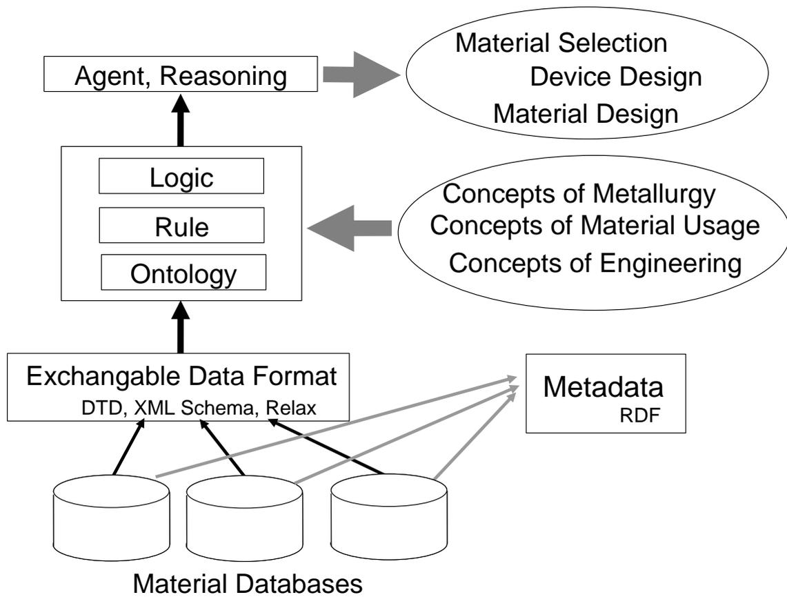
**Figure 1.** Material databases and Semantic Web technology
