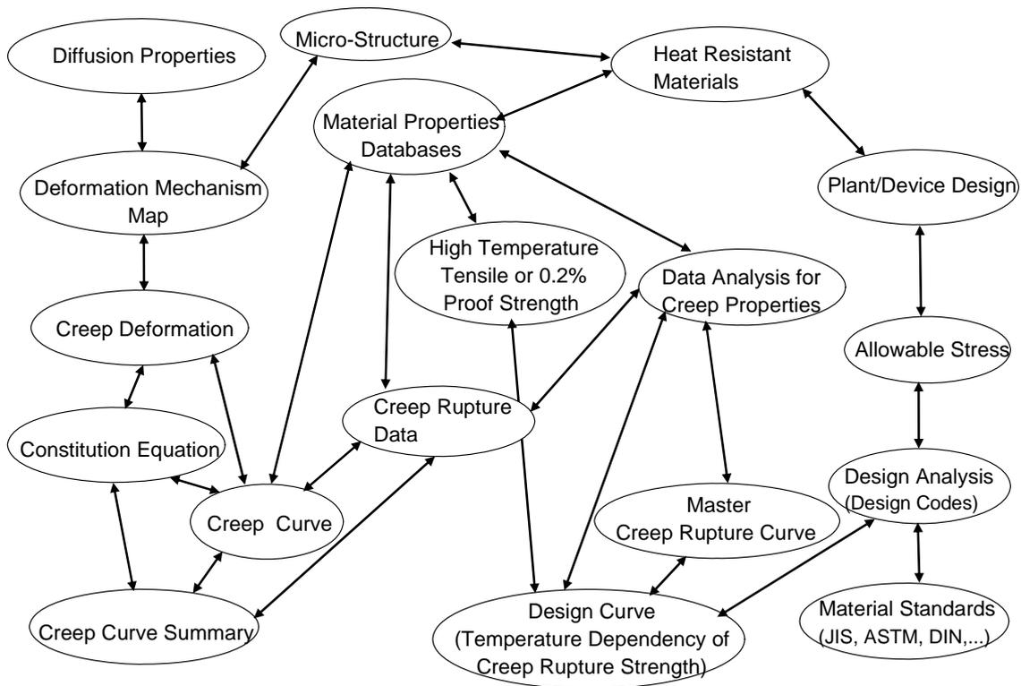
Figure 5. Standard procedure to derive a design curve from a creep data sheet
