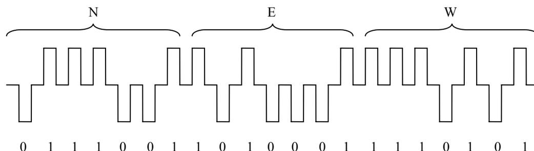
**Figure 2.** Hybrid data telecommunication system digital bit-stream with the adopted  $k=7$ ,  $M=128$ , code
