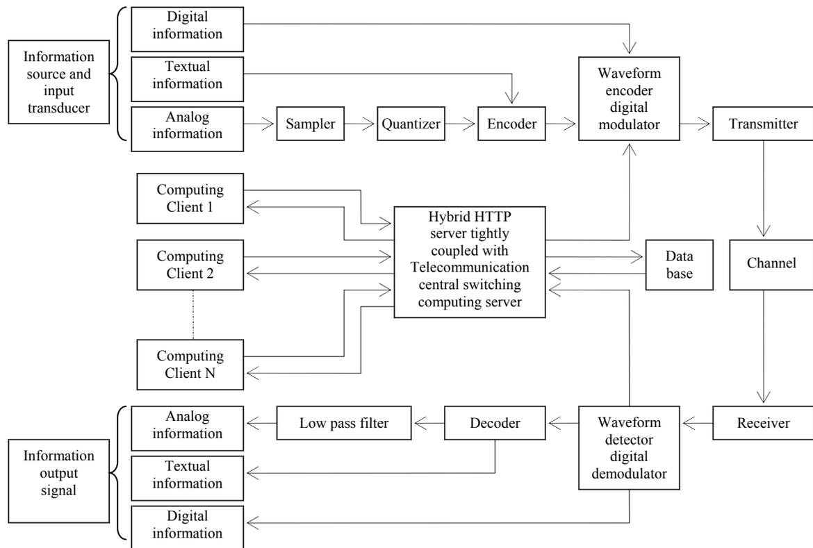
**Figure 1.** A polythematic real-time hybrid data telecommunication system for scientific research
