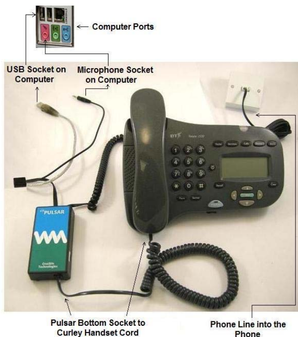
Figure 1. Pulsar Plus recording equipment, showing the break in the telephone circuit and the computer connection
