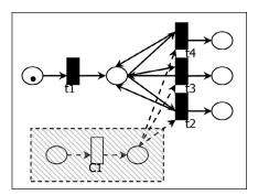
Figure 5: The selective structure with choice conditions.
