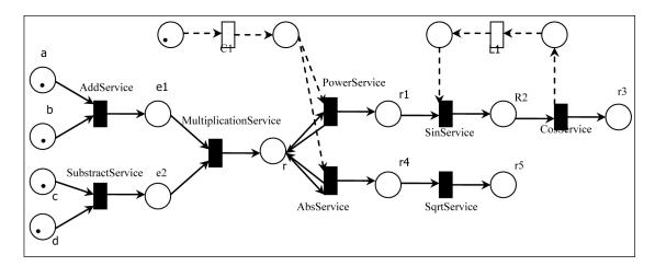
Figure 6: Scientific computing service Petri net.
