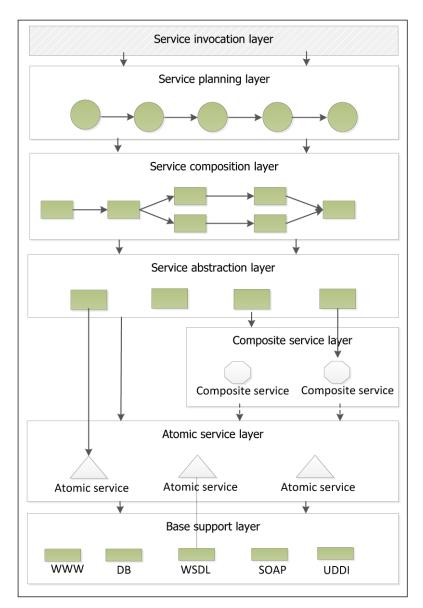
Figure 2: The layered service composition architecture.
