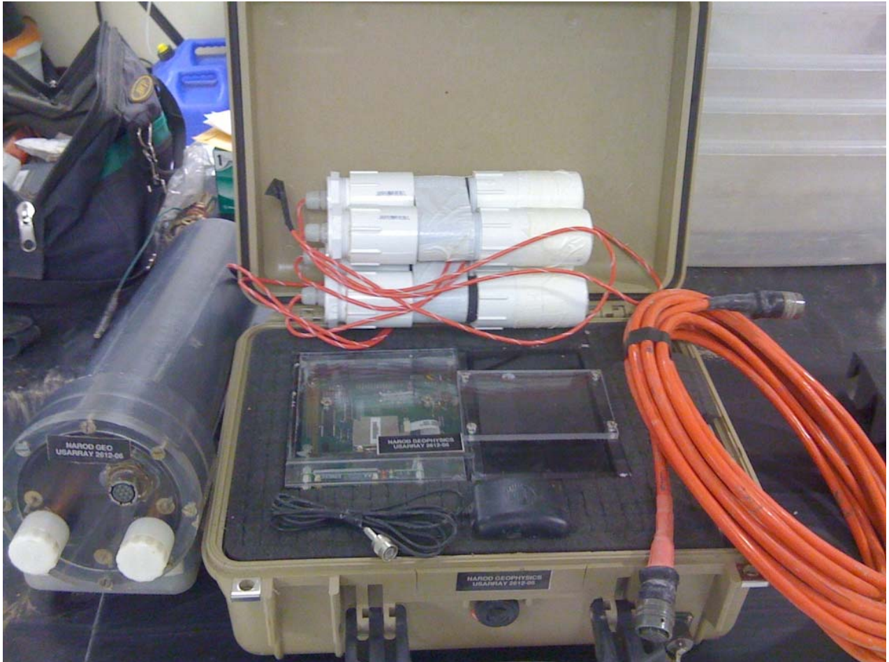
Figure 1. Transportable MT Array field equipment. Triaxial ring core fluxgate magnetometer sensor (left), data acquisition system (center), non-polarizing Pb-PbCl 2 electrodes (center, top). 2-3 week instrument deployment yields data in period range of 10 s to 20,000 s. Longer periods -> deeper penetration into Earth's interior.
