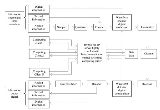
Figure 1. A polythematic real-time hybrid data telecommunication system for scientific research
