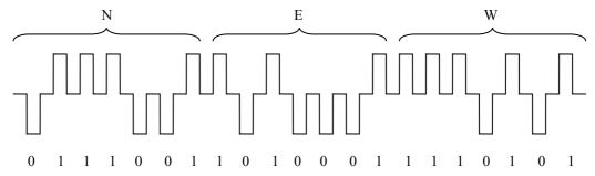
Figure 2. Hybrid data telecommunication system digital bit-stream with the adopted k=7, M=128, code
