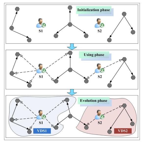
Figure 2: The working principle of VDS in different stages.
